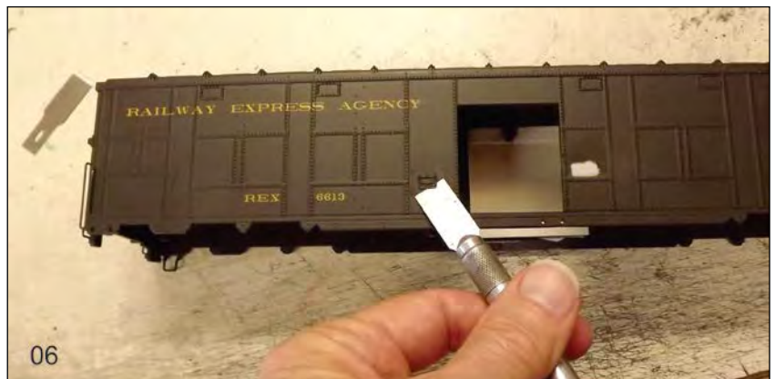
Paint was scraped down to bare ABS at the new location for the cardholder, gauged from prototype photos.
