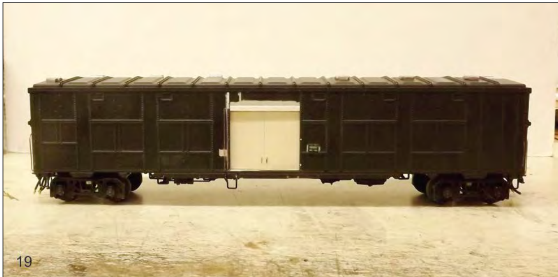
Right side handrail holes were plugged with styrene rod. Handles were added to the doors. The original doorway handrail was moved to the left side.
