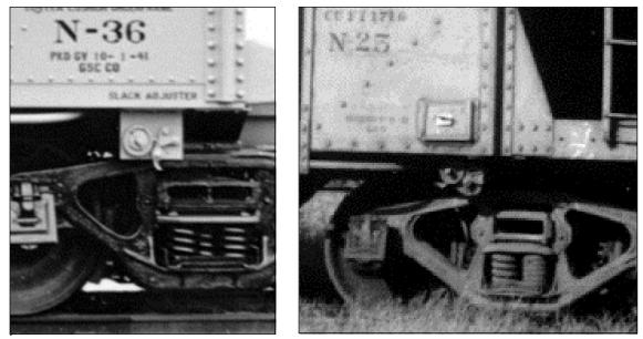
Figure 3 – (Left) The XLT slack adjuster applied to class N-36 covered hopper. Note that this is a mirror image of the version shown in figure 1 above. (Right) The XLT on the N-25 has a slightly different back plate.
