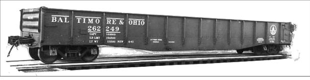
Figure 2 - 0-59A number 262249 clearly shows the XLT Slack Adjuster below the fifth stake from the left (A) end. Photo courtesy of Bob Witt, BORHS.
