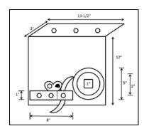
Figure 4 - Line diagram of the ratchet assembly common to both types of XLT Slack Adjusters. Dimensions in scale inches. Chris Tilley diagram, based on application seen on M-53 385897 at The Baltimore & Ohio Railroad Museum. The gear has 28 teeth and is 5 inches across. The washer is 3 inches across. The shaft is 1-3/8 inches (round) coming out of the back of this assembly, and 1 inch square on the visible end. Covered hopper applications are mirror images of this diagram.
