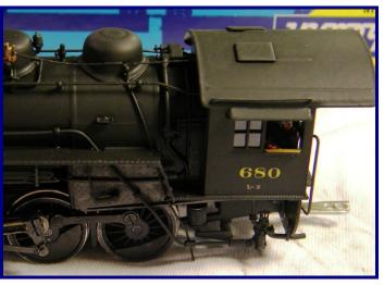
The lift bar and coupler head are connected with fine blackened chain. The windows are glazed, with the "glass" held in place with white glue. Someday I want to try using microscope cover glass (slide covers).
