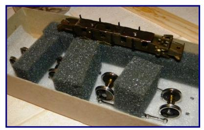
Segregate and label all parts for ease in reassembly. Draw a diagram of especially difficult assemblies.
