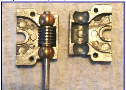
Gearbox cleaned and additional thrust washers installed. In this photo the thrust washers are added on either side of the worm. The new washers were ultimately mounted outside the stock thrust washers.
