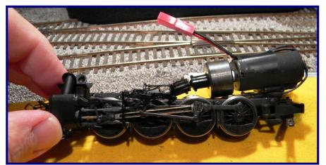
Locomotive frame with NWSL motor and connector parts. This assembly was bench tested several times for 30 minutes each, in forward and reverse, to ensure no surprises when the locomotive is complete.
