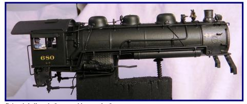
Painted shell ready for assembly onto the frame.
