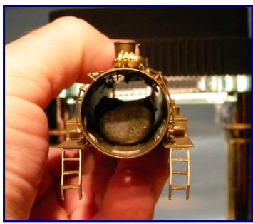
blob to the joint. As the flux evaporates, the solder is Boiler weight is filed down to allow plugs and wires to pass to the drawn in quickly and solidifies almost instantly. Make headlight. Locomotive still has plenty of weight for pulling. sure to take appropriate safety precautions when soldering. Practice with some non-critical parts first. Some filing
