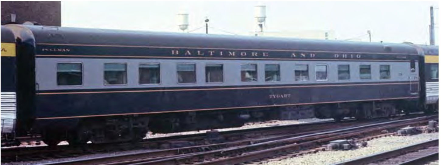
5-3 Tygart was a 10-roomette, 6 double bedroom sleeper from a group built in 1951.
