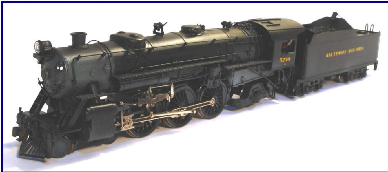
Very minor modifications were required to this brass Akane USRA 4-6-2 to capture the appearance of the B&O engine. The headlight was raised from the center of the smokebox to the high position and a Cal-Scale B&O Capitol plate was installed at the center of the smokebox. The USRA trailing truck was replaced with a Delta truck kit from Precision Scale. Last, an engineer and fireman were added to the cab. Class P-6A used both USRA and Vanderbilt tenders,
