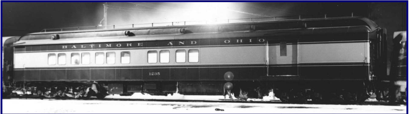
B&O 1235, Class D-14AB, Willard OH, December 18, 1964 (E. J. Wolford photo). Originally Class D-14 #1421 built October 1917, rebuilt into Class D-14A June 1936, rebuilt into Class D-14AB June 1941 and renumbered #1235, retired 1969.
