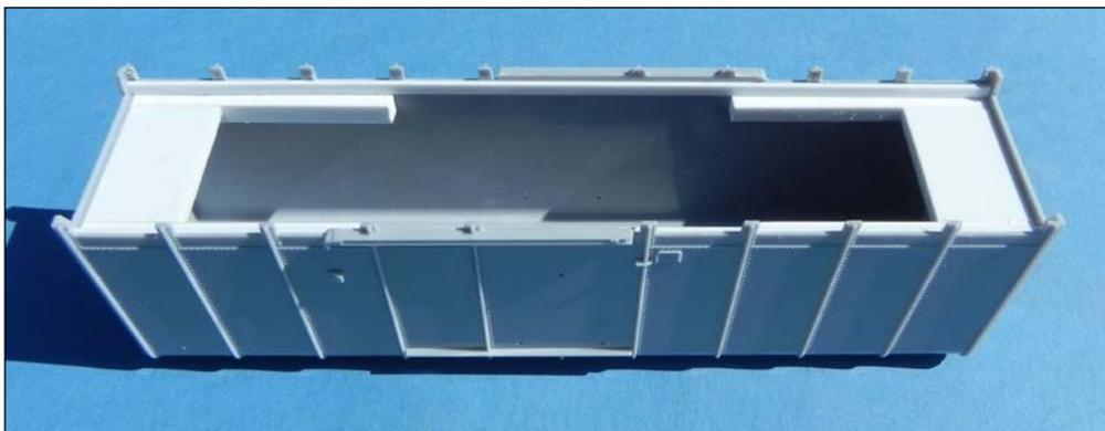
I substituted .040" x .080" sidesill spacers in place of the .040" x .100" strips
