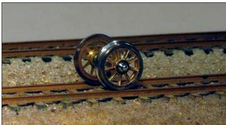
The brass truck required some re-soldering and filing to get it to fit under the Bachmann model. I also added some shaped lead under the truck to ensure the truck would track well.
