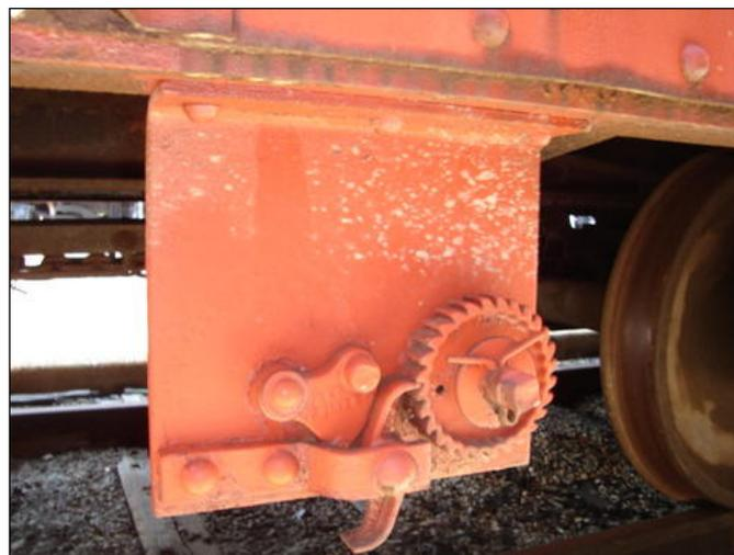
Figure 1 - XLT Slack Adjuster ratchet mechanism as applied to M-53. Chris Tilley photo.
