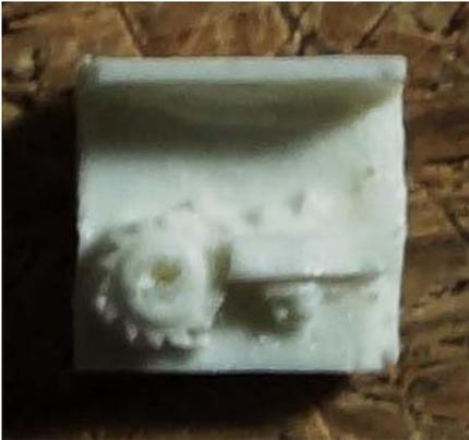
Figure 5 - Chris Tilley's scratchbuilt resin casting (about 10x life size in the photo) of the XLT Slack Adjuster for covered hopper applications.
