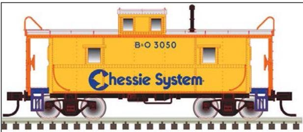
**Atlas** is releasing an HO-scale steel caboose with centered cupola and equipped with Accumate knuckle couplers. The Trainman series ready-to-run model is based on a prototype Magor Car Co. car built in 1937 for the Chesapeake & Ohio. In addition to the C&O, road names will include B&O Chessie System. For additional information, contact a dealer or visit the [announcement page](#).
