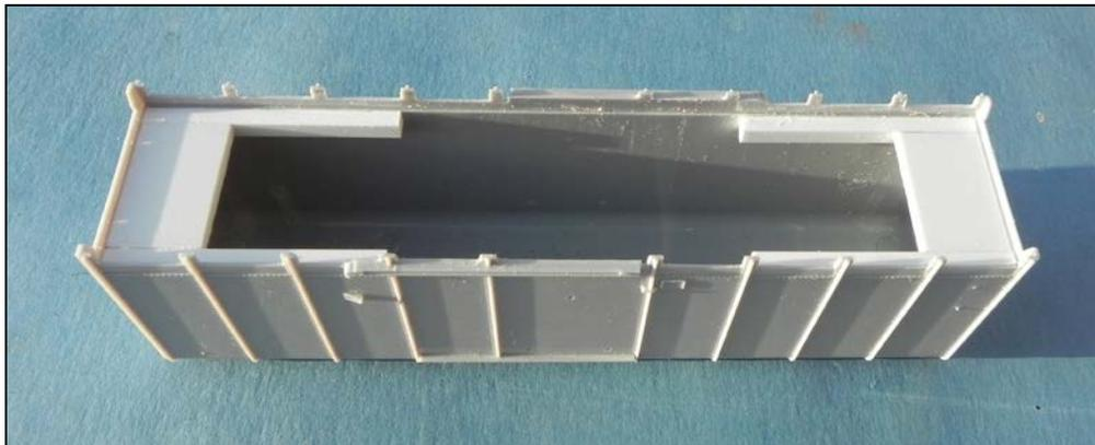
The floor is supported by .125" x .125" strips and .080" pads.
