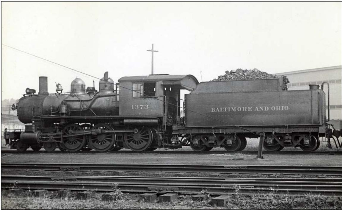
Another nearly left broadside, again of 1373 taken at Clarksburg, WV in July 1939. The new steel cab has a hood at the rear where they hung winter curtains. The squared off driver counter weights are really visible here with the side rods in the upper position. Malcolm McCarter photo.
