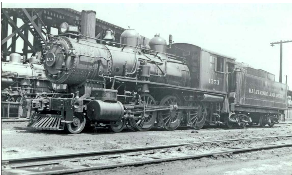
The subject of my model 1373 is shown here at Parkersburg, WV on August 11, 1940. It is one of the B-8 class built by Baldwin Locomotive Works in 1893, now modernized with electric headlight, steel cab and larger tender. According to *Steam Locomotives of the Baltimore & Ohio, An All-Time Roster* by William D. Edson, 1373 was scrapped in August of 1947. Edwin Kirstatter's Collection.
